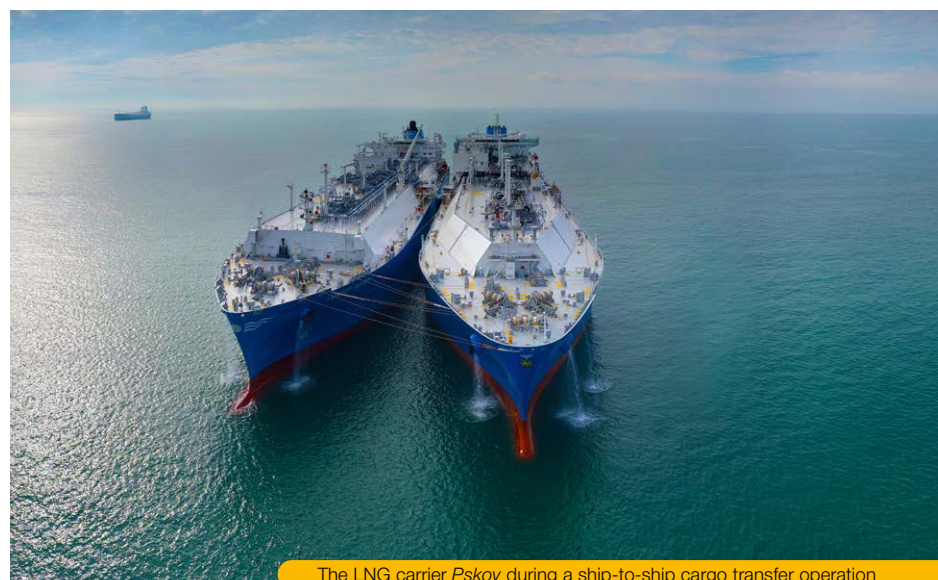
The LNG carrier Pskov during a ship-to-ship cargo transfer operation
